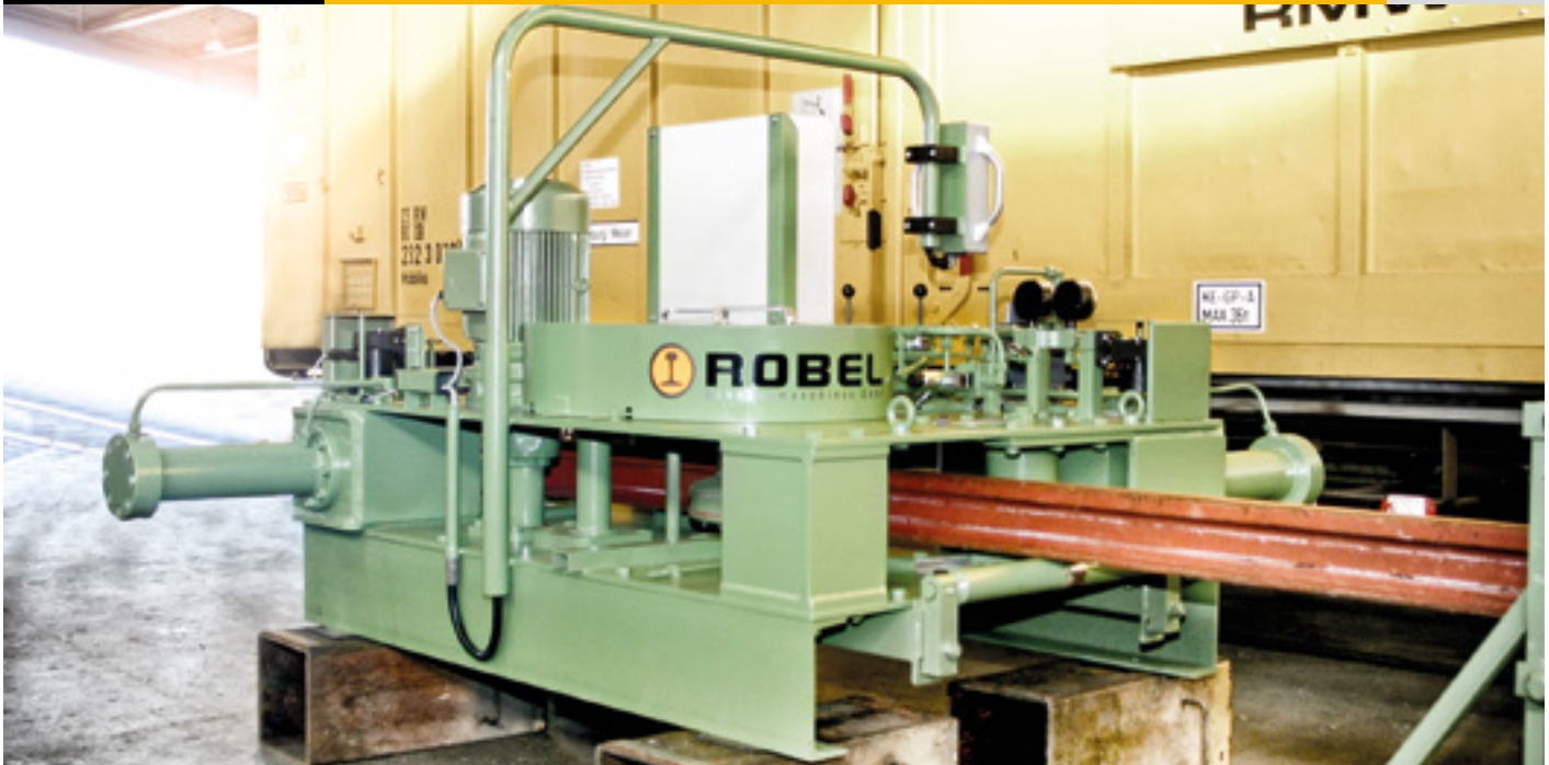
4 Roller-type Rail Bending Machine with hydraulic (roll) feed for bending grooved rails and vignol rails.
