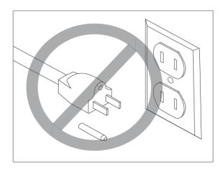
This equipment must have a ground prong in the plug to help ensure that it is grounded. DO NOT remove ground prong from plug to fit into a two-pronged outlet! If the plug will not fit the outlet, have the proper outlet installed by a qualified electrician.
