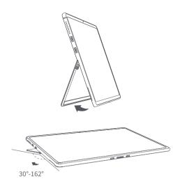
⚠To prevent damage kickstand hinge, do not apply excessive pressure to the kickstand!
