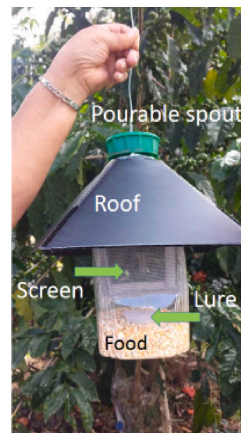
Fig. 1. The breeding station components. Cathartus quadricollis adults are attracted to the aggregation pheromone (quadrilure), and pass through the screen into the station and find the food. The food and lure are inserted through the spout, and the roof helps keep the food dry.
