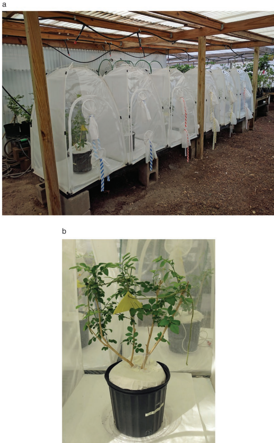
Fig. 2. (a) Cages used for greenhouse trials with D. citri adults and (b) AK device on a potted orange jasmine plant.
