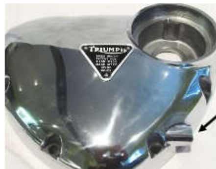
Figure 3 - Triumph timing cover with oil pressure access hole
