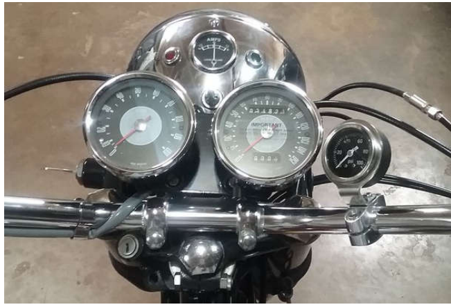
Figure 1 - Triumph oil pressure gauge kit installed on a 1970 Triumph T120R
