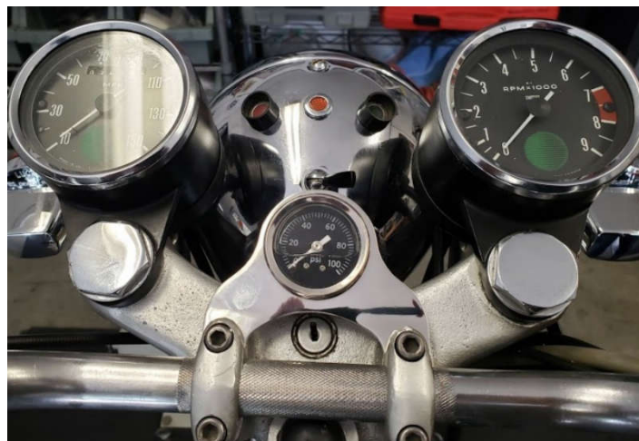
Figure 4 - Norton oil pressure gauge fitted to a Norton Commando MK2
