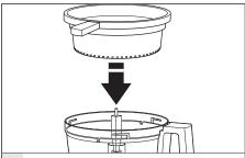
Place the strainer basket in the work bowl with the locking clip positioned to the left of the work bowl handle.
