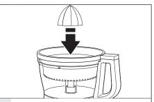
Place the cone inside the strainer basket, over the power shaft. It may be necessary to rotate the cone until it falls into place.
