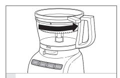
Turn the basket counter clockwise until the clip locks into the handle.
