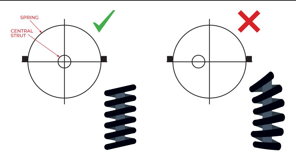
N.B. As the central shaft of the strut is offset on a lot of modern vehicles, care must be taken to ensure that the offset shaft is centralised prior to compression. Misalignment will make compression more difficult.
