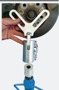
Allows the suspension axle to be raised and lowered to the required position using a hydraulic jack.
