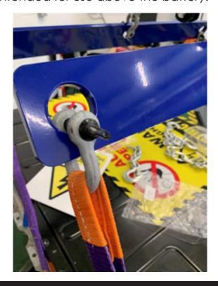
• Sufficient shackles are supplied to allow each of six lifting slings to have a shackle at either end. However, it may be preferable to fit two slings to one shackle as shown here.
