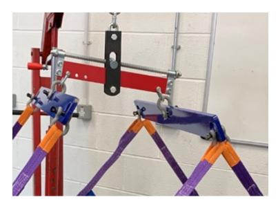
• At the top of the leveler a 1.5 ton shackle is used to attach to the pick-up point.
