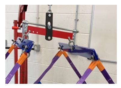
• The two shackles shown here attached to the red arm of the leveler should be the 2-off 0.75ton rated supplied with the kit not those supplied with the leveler (as illustrated here)
