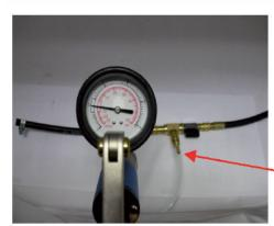
Adaptor fits into tap connector allowing connection of a vacuum gauge/pump. Connections to vehicle as for pressure fed systems
