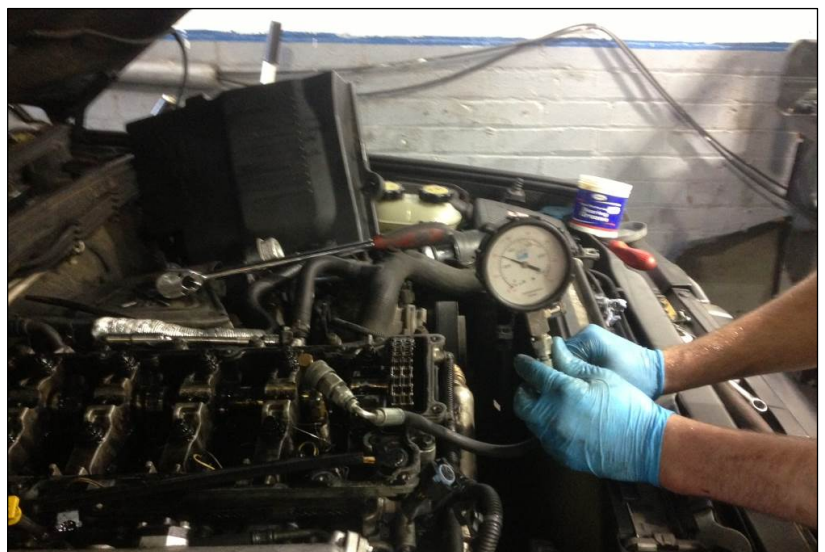
Image shows testing a TD5 engine with 31424700 connected to an old SP Pressure Gauge
