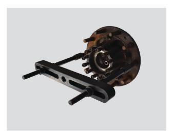
3. Fit nuts (part 4) onto each rod (part 3). Slide beam down to meet nuts and secure with remaining 2 nuts on top of the beam.
