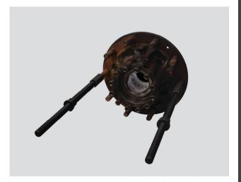
2. Fully screw pulling rods (part 3) into adaptors (parts 5 - 9).
