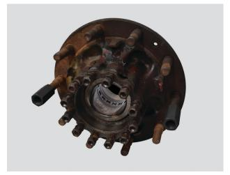
1. Fully screw on correct adaptors to suit wheel studs from parts 5 - 9.
