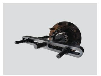
4. Insert axle end plug (part 10, 11 or 12). Insert and turn screw (part 27) to meet axle plug and turn to remove hub. Take care with this step due to the weight of the hub. Ensure pull is slow and gradual. All threaded parts are to be greased before use.
