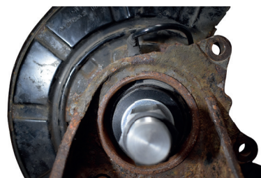
ABS sensor shown with clearance
