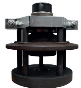
Removal of inner race can be done with workshop press or spindle and nuts
