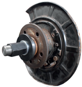
Installation of the wheel hub flange
