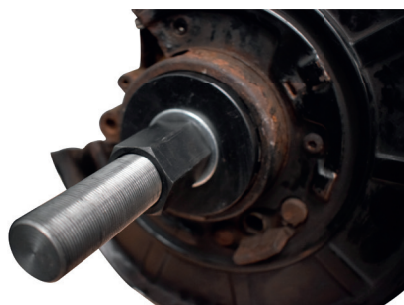
Installation of new bearing
