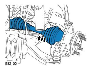
CAUTION: Do not allow halfshafts to hang unsupported at one end or joint damage will occur.
