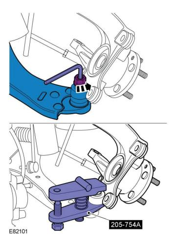
WARNING: Make sure that a new lower arm ball joint nut is installed.
