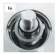
Ensure stub shaft is bottomed completely on motor shaft and torqued.
