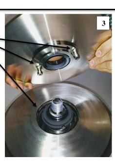
Place O-ring on shaft and thread on impeller
