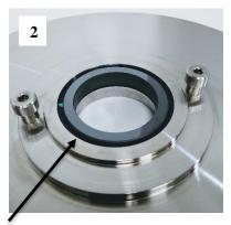
Stationary silicon carbide seal in Viton cup
