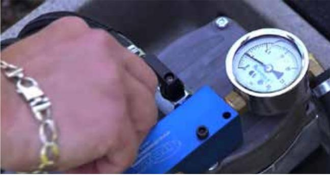
Bubbles should be noticeable on the pond's surface from the diffuser locations. When more than one diffuser is installed, adjust the airflow valves on the compressor manifold (For Option B with Remote Manifold, do this step at the remote manifold). Once an adjustment is made, you may need to wait several minutes to see the results at the diffuser location(s).
