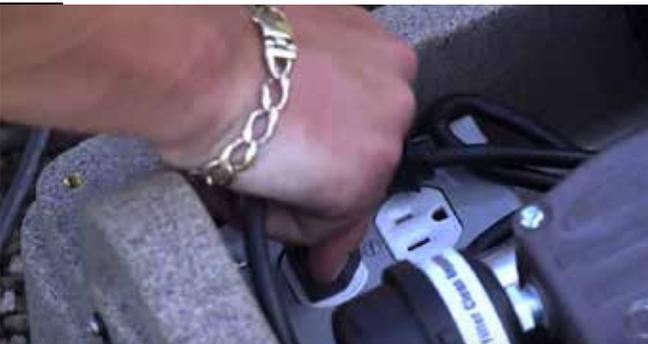
**PS10 Systems:** Plug the compressor and cooling fan into the power control outlet inside of the cabinet (Fig. 1). Plug the cabinet power cord into a GFCI power outlet.
