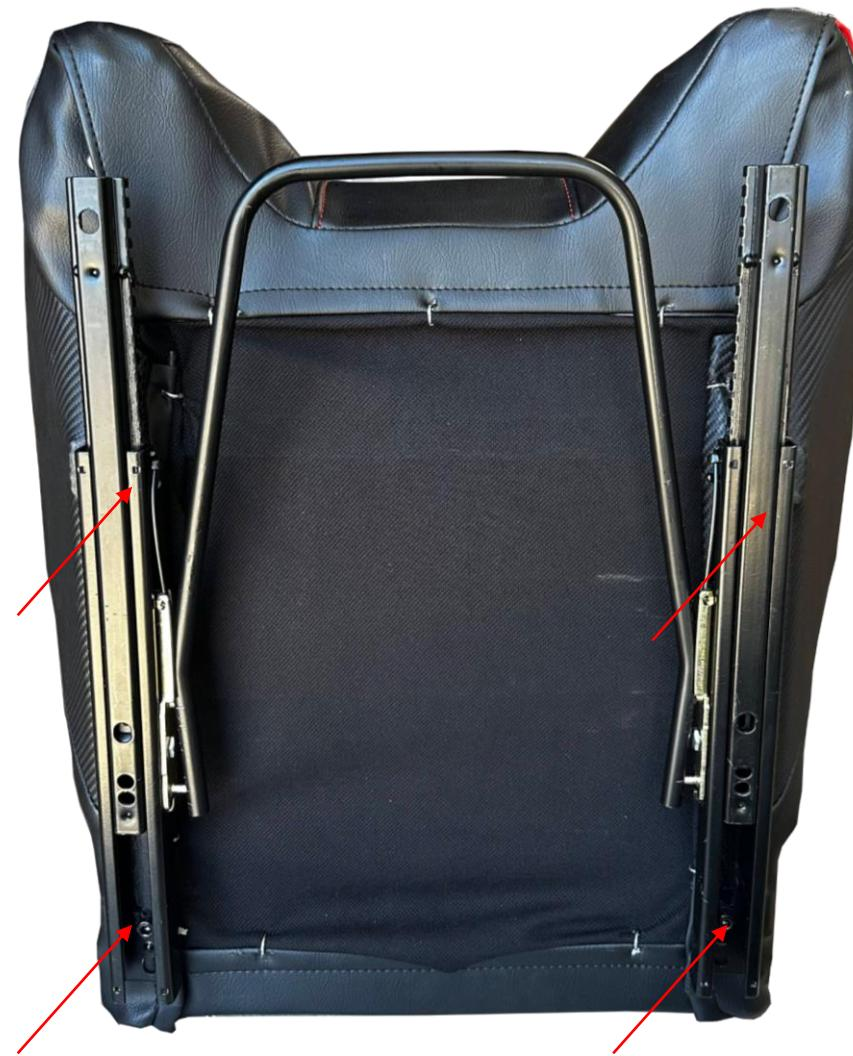
Install seat slider under the seat
