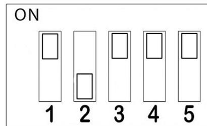
**Buffered Bypass w/ Delay Trails**
