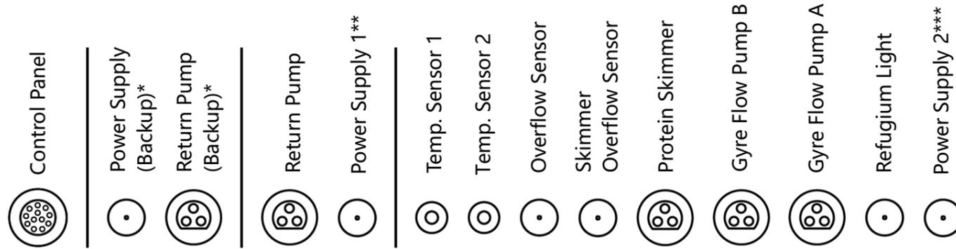
\* Tips: When the main control system is failed, please first connect the Return Pump and Power Supply 1 to the Return Pump (Backup) and Power Supply (Backup) sockets respectively, now the Power Supply 1 only powers the return pump, the other equipment stops working. Then please contact local retailer or manufacturer for after-sale service.
