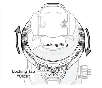
Figure 12. Secure Locking Ring
