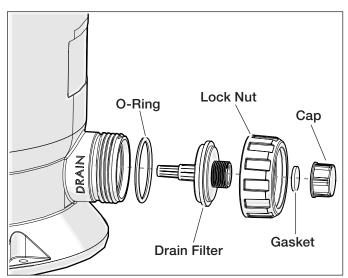
Figure 8. Drain Cap
