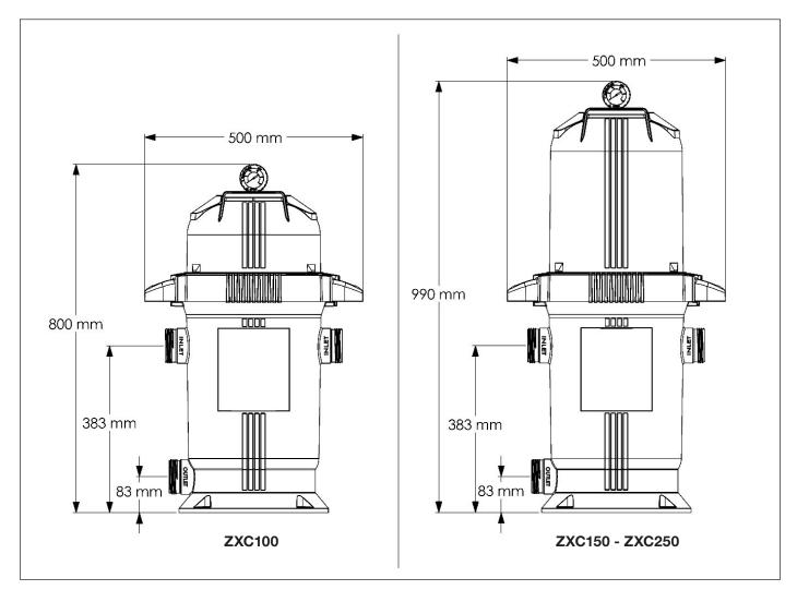
Figure 1. ZXC-Series Filter Dimensions
