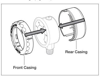
Figure 9. Pressure Gauge Casings
