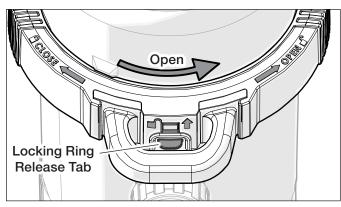
Figure 15. Locking Ring Release Tab
