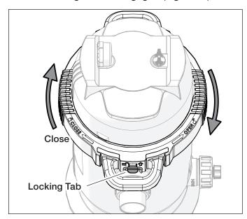
Figure 18. Closing the Locking Ring
