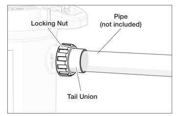
Figure 5. Plumbing Connections
