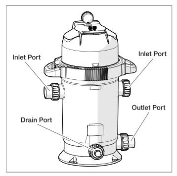
Figure 4. Filter Ports
