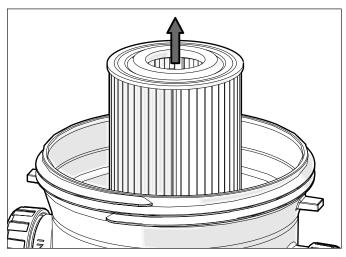
Figure 16. Removing Cartridge
