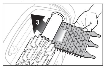
Figure 25. Install the New Brush
