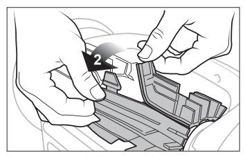
Figure 24. Undo the Tabs of the Brush
