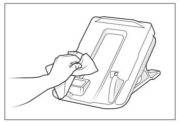
Figure 18. Clean the Charge Plates
