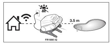
Figure 17. Charging Station Distance to Pool Edge
