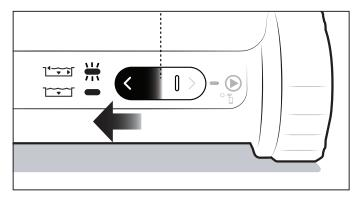
Figure 7. Slide and Release Left to Select Mode
