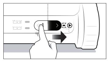
Figure 8. Slide and Release Right to Start
