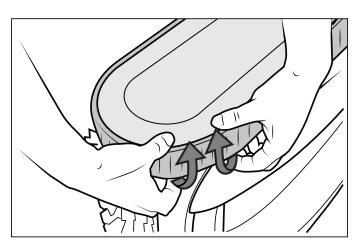
Figure 28. Pull the Old Track Over the Wheel
