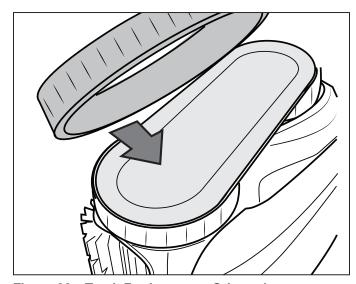
Figure 30. Track Replacement Orientation
