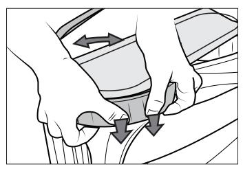
Figure 33. Push the Track into Place on the Wheel
