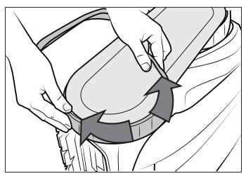
Figure 32. Work the Track On Around the Wheel
