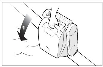
Figure 9. Submerge the Cleaner Vertically
