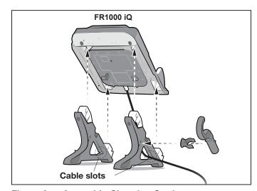
Figure 2. Assemble Charging Station
