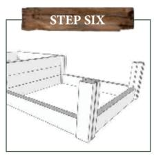
If your raised bed has 2 or 3 bays, there is a bit more to do... Take two more boards and using the posts on one of the completed sides of the raised bed, slide in the bottom board at the front and back.
