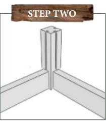
Insert one side board and another board at the front by sliding the end of each board evenly into the appropriate post slot.
