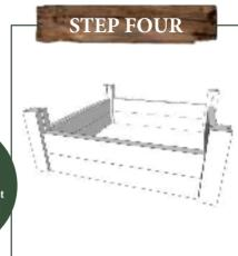
Ensuring that from the front and from the back the unmachined side of the post faces you, use three more posts and two more boards to build a square – simply slide the boards into the posts as before.
