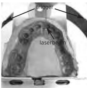
Turn the unit on at the main switch at the unit's front (a green control is lit). Activate the laser by pressing either one of the triggers. Align/determine the drilling position by means of the laser beam.
