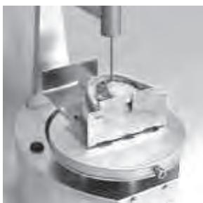
Place the plate support with impression carrier onto the magnetic table.
