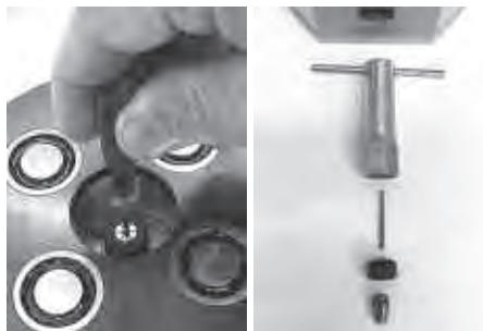
The burr rests on a slotted screw in the center of the axis. Clockwise turns lower the screw = tighter drill hole; counter-clockwise turns raise up the screw = wider drill hole. The wider the drill hole, the farther the pin tip juts out of the plinth plate.
