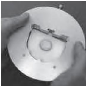
Insert the plinth plate into the plate support from the bottom. First, press the frontal groove of the plinth plate against the spring bolt; then have the dove-tail engage at the opposite side. Tighten the fixing screw by hand.
