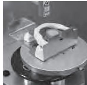
Both metal nozzles on top of the plate support clutch the two drill holes of the impression carrier.
