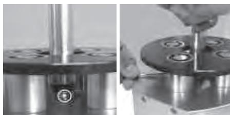
Unplug the power cable. Insert the fixing pin from the side into one of the holes of the drilling axis. Turn the tubular socket wrench in counter-clockwise direction to unscrew the sleeve nut. Then, remove the defective burr.
