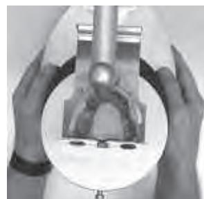
Pressing of both triggers at the same time automatically fixes the plate reception and initiates the drilling process.
