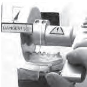
Fix the plinth plate in the model table of the DIACUT model saw (171800). Align the model table in accordance with the cutting direction. The saw cuts as defined.
