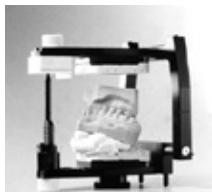
Once plaster has set, pull out magnetic part with knurled handle with a twisting movement. Open mounting articulator. Remove maxilla from impressions. Remove transference from the mounting articulator.
