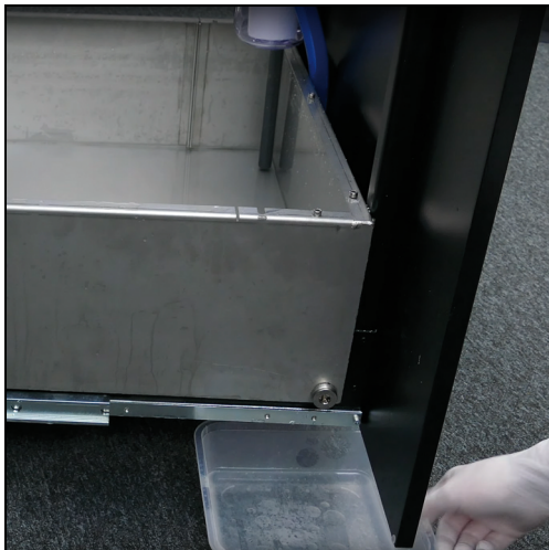
11. Place suitable collection container under tank drain plug.
