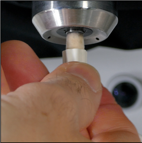
6. Clean collet with felt cone [2].
