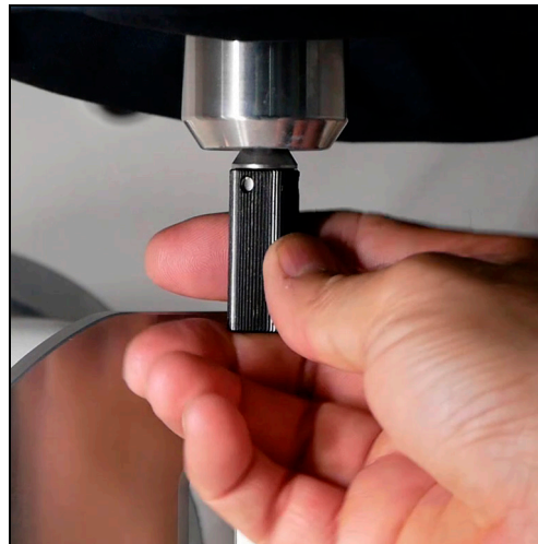
12. Tighten collet until torque wrench "clicks".
