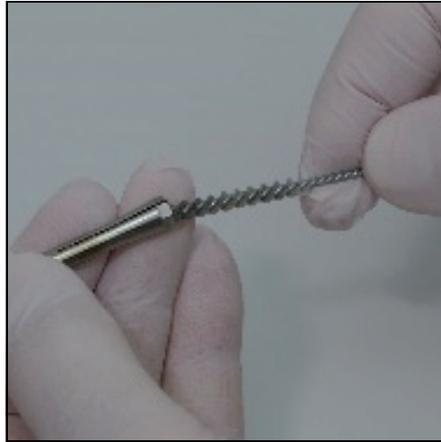
7. Clean collet cone with collet brush [4] from both sides.
