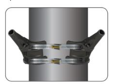
With a 5/16 drill bit or a flat head screw driver, tighten the assembly around the pole to ensure the kit does not come loose.
