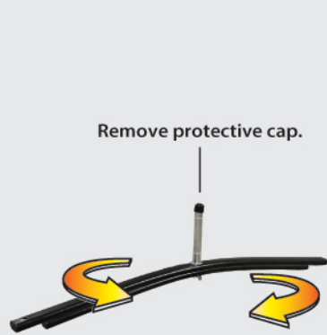
Rotate upper and lower arms to create X shape.
