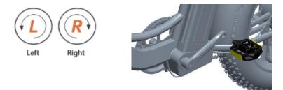
(2) Tighten the right pedal "R" clockwise, Tighten the left pedal "L" counterclockwise.
