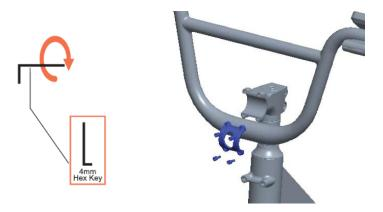
(2) Install 4mm hexagon wrench clockwise. Do not tighten the 4 bolts in FIG. A. Adjust the handle to the proper Angle in Fig. B, and then tighten the 4 bolts with proper force.
