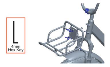
(2) Install 4 bolts clockwise using a 4mm hexagon wrench, and place the harness in the front shelf hook.
