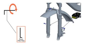
(2) The mudguard support shall be aligned with the front fork mudguard take-up hole position, and then threaded into the screw for tightening.
