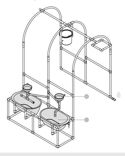
**Important:** Please ensure that all connections are tight before attaching a hose. If water leaks occur, you will need to tighten the connections by pushing them together or using a rubber mallet to bang them closed.
