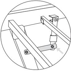
Straighten the hinge and secure the legs structure by moving the security caps down.
