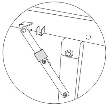
**⚠WARNING: FALL HAZARD.** Always place security caps in place around leg hinge before use. Failure to do so may lead to serious injury.
