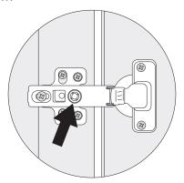
(D) FOR VERTICAL ADJUSTMENT LOOSEN THE INDICATED SCREWS, ALIGN AND TIGHTEN.
