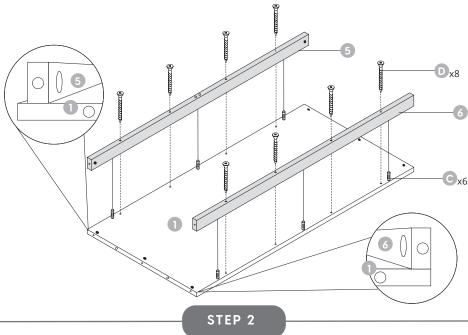
SECURE THE BACK RAIL (5) TO THE BOTTOM PANEL (4) USING DOWEL PINS (C) AND LONG SCREWS (D).
