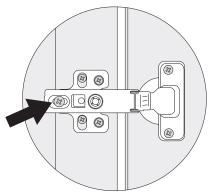
(C) FOR FORWARD AND BACKWARDS ADJUSTMENT, USE THE SCREW INDICATED BELOW.
