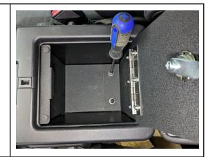
For the best fit, hold the panels in place while tightening down the screws
