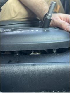
Reinstall the shifter knob. Give it a good hit to snap it into place.
