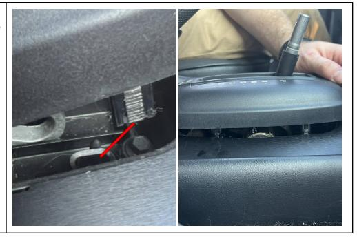
Reinstall the shifter knob. Give it a good hit to snap it into place.
