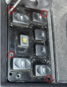
Remove the 4 clipnuts from the tabs..
