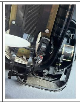
Reinstall the shifter boot. Be sure to line up the tabs with the holes.
