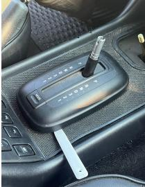
Pull the boot straight upwards to release.
