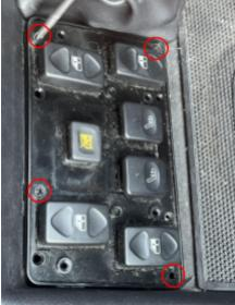
Remove the 4 clipnuts from the tabs..
