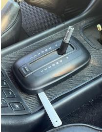
Pull the boot straight upwards to release.
