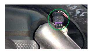
7.) Pull the electric cable of the exhaust flap control unit up to the exhaust flap. If necessary, you can also hide the electrical cable under the heat shield. Usually a few small screws have to be removed and reattached later.
