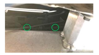
11.) Identify the exhaust flap electric actuator on the right side. It is located on the right side above the rear silencer (green circle). On some models, the servomotor can also be located behind the rear silencer.
