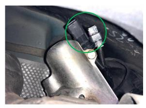
8.) Now connect the plug that was separated from the exhaust flap to the matching socket of the exhaust flap control unit until it snaps into place (1). Then slide the gray lock of the plug towards the socket so that the plug can no longer be detached (2).
