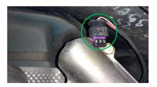
7.) Pull the electric cable of the exhaust flap control unit up to the exhaust flap. If necessary, you can also hide the electrical cable under the heat shield. Usually a few small screws have to be removed and reattached later.
