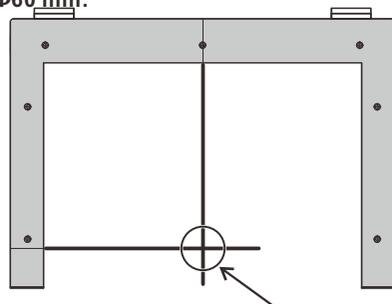
Foro passacavi  $\Phi 40 \sim 60 \text{ mm}$
