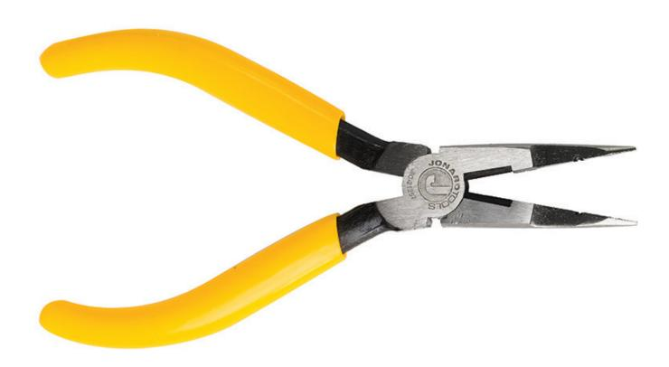
Jonard's long nose pliers are made of heat treated chrome vanadium steel with induction-hardened cutting edges for maximum strength and durability. These long nose pliers feature the following:
