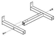
Note: The channel nut teeth should always face towards the bolt head.  $\stackrel{ extstyle of }{=}$
