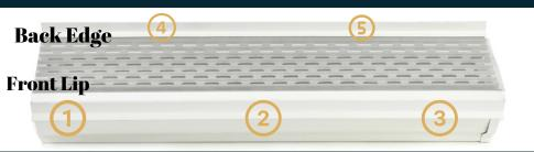
The tab on the left end of each panel installs under the adjoining panel. Use screw holes along the front lip of Leaf4go Micromesh to zip screw the panel - 3 or 4 screws (1, 2 & 3) to the front lip of the gutter and 2 screws for the back (4 & 5). DIAGRAM 2: Shows recommended cuts for connecting inside corner pieces together.
