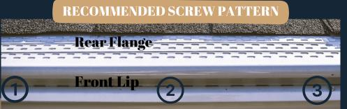
The tab on the left end of each panel installs under the adjoining panel. Use screw holes along the front lip of Leaf4go gutter guards to zip screw the panel - 3 or 4 screws (1, 2 & 3) to the front lip of the gutter. DIAGRAM 2: Shows screw holes along the front lip of Waterlock Pro.
