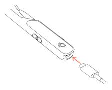
2 Plug the larger end of the USB charging cable into a standard USB wall adapter [5W/5V/1A] (not included).
