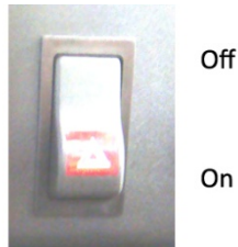
Hazard Light Switch
