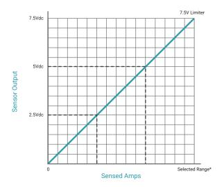
\*Factory calibrated ranges selected with the amperage range switch
