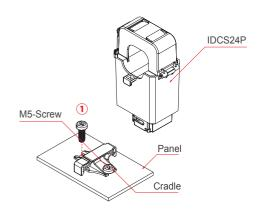
Place the cradle on the Panel and fix it via M5 screw.
