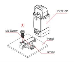
Place the cradle on the Panel and fix it via M5 screw.
