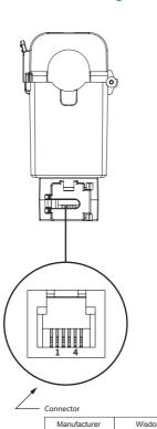
This product needs  $\pm 15V$  (+15V and -15V DC bi-polar power supply) as operating power supply. Even if the case of current detection of only plus direction,
