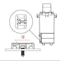
Install the product on the cradle, while matching the arrow direction of cradle and indication in the bottom of the product.
