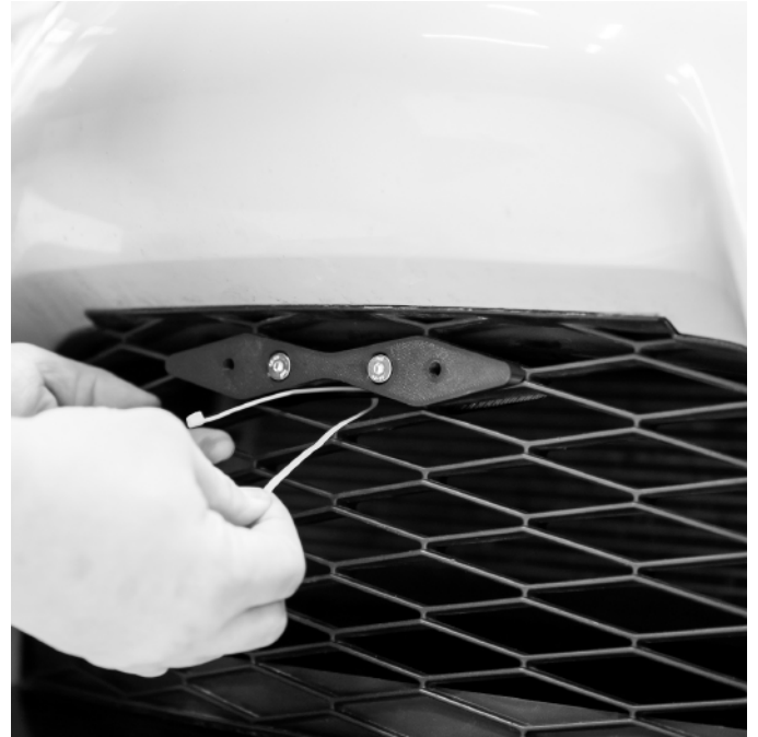
*For removal insert tie-wrap as pictured and reverse the installation process.
