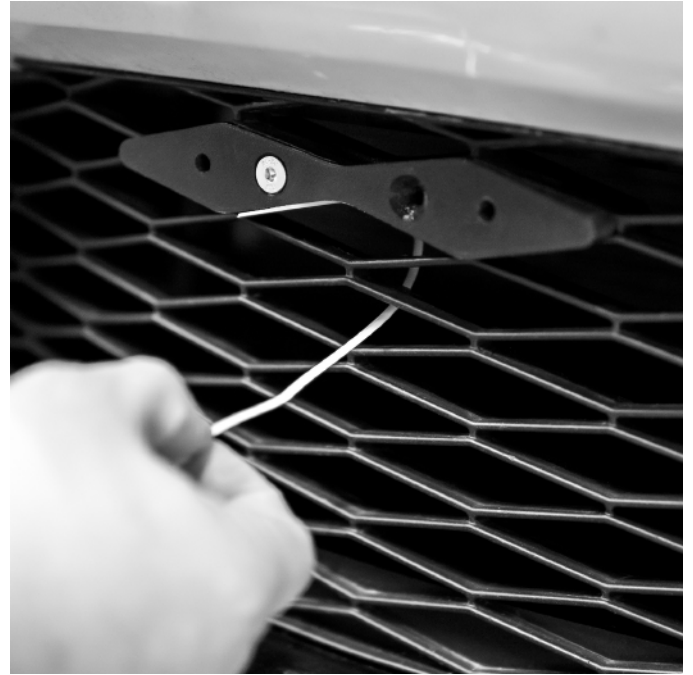
6. Remove tie-wrap and & install 2nd bolt. Do not over tighten bolts.
