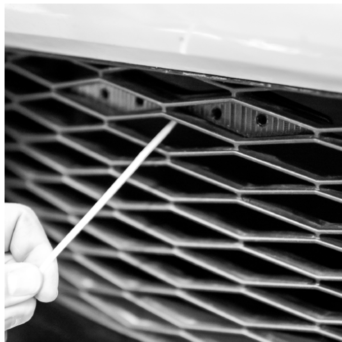
4. Use tie-wrap to assist in placement
