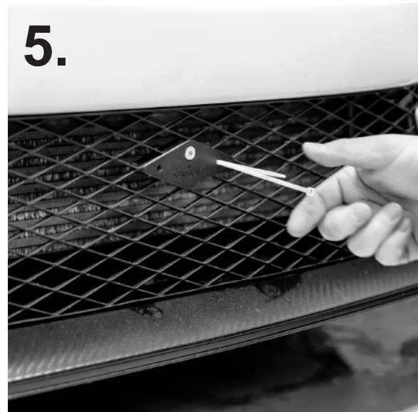
5. Install the M6x25mm bolt (Do not over tighten) and remove zip-tie
