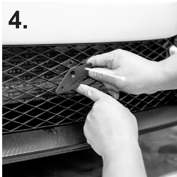
4. Once inserted align the back and front plate into install position.
