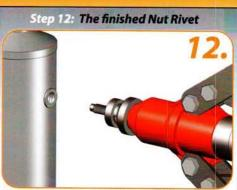
The nut rivet should now be securely in place and unable to turn.
