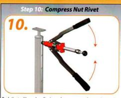
Push the tool lever handles inwards to compress the nut rivet against the wall of the tube. This will fasten the nut rivet in place.
