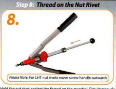
Hold the nut rivet against the thread on the mandrel. Simultaneously push the screw handle inwards. Pushing the screw handle inwards will thread the nut rivet on to the mandrel.
