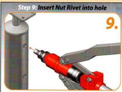
With the nut rivet on the mandrel of the tool insert the nut rivet in to the pre-drilled hole.
