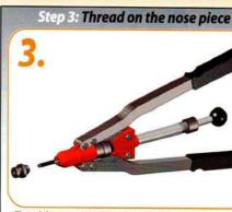
Insert the mandrel (threaded end first) in to the body of the tool. Replace the screw handle using the screw handle retaining nut. Thread the nose on to the main body of the tool. The nose piece being used must match the size of mandrel being used. Ensure the nose piece locking nut is on the nose piece before threading on.
