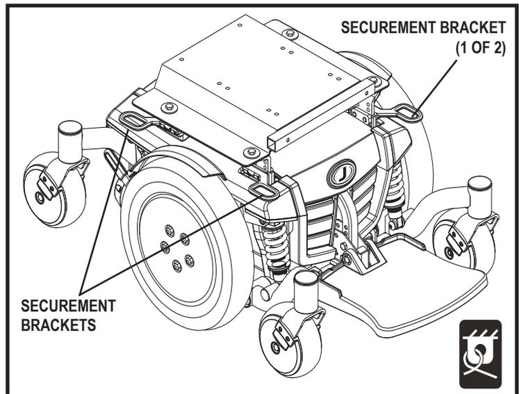
Figure 13. Transit System Securement Brackets-UK Occupied Transit
